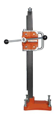
Core drill rig KBS-252/Light-K
